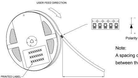
A spacing of approximately 160mm between the front edge of tape
